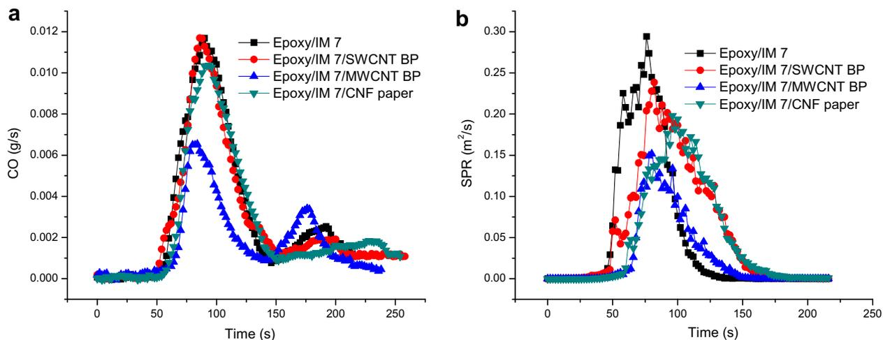
Fig. 5 – Comparison of CO production rate (a) and smoke production rate (b) during combustion.
