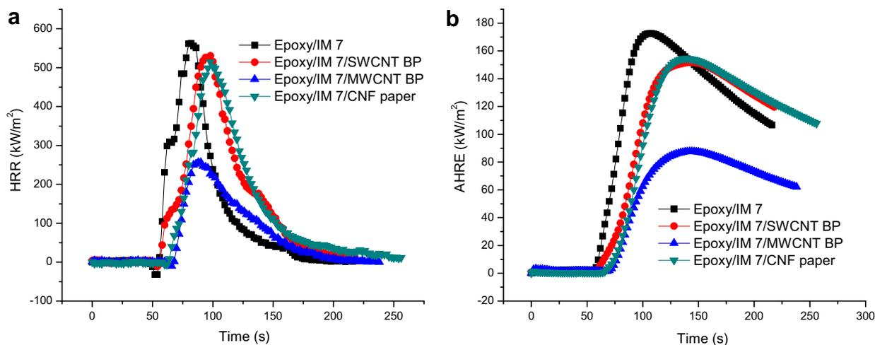
Fig. 4 – Comparison of heat release rate curves and average rate (a) of heat emission curves (b) for Epoxy/IM-7, Epoxy/IM-7/SWCNT-BP, Epoxy/IM-7/MWCNT-BP and Epoxy/IM-7/CNF paper.
