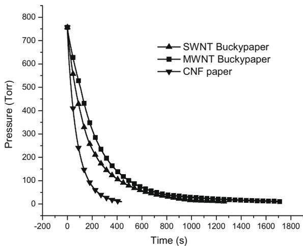
**Fig. 3 – Pressure drop curves of gas flow through SWCNT buckypaper, MWCNT buckypaper and CNF paper.**
