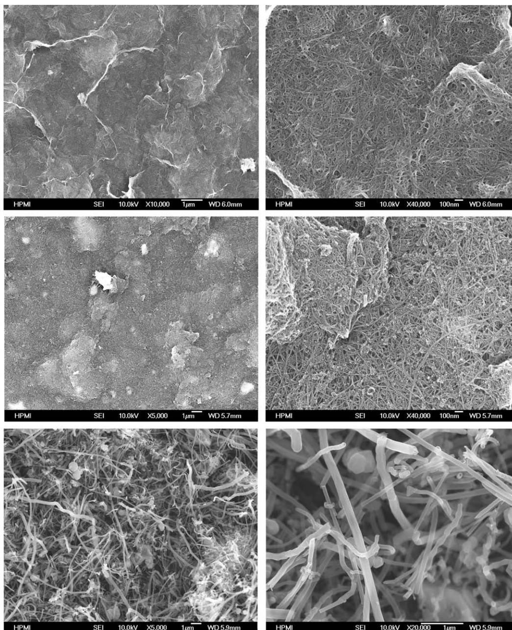
**Fig. 1 – SEM images of SWCNT, MWCNT buckypaper and CNF paper (from top to bottom). Left: low magnification; right: high magnification.**
