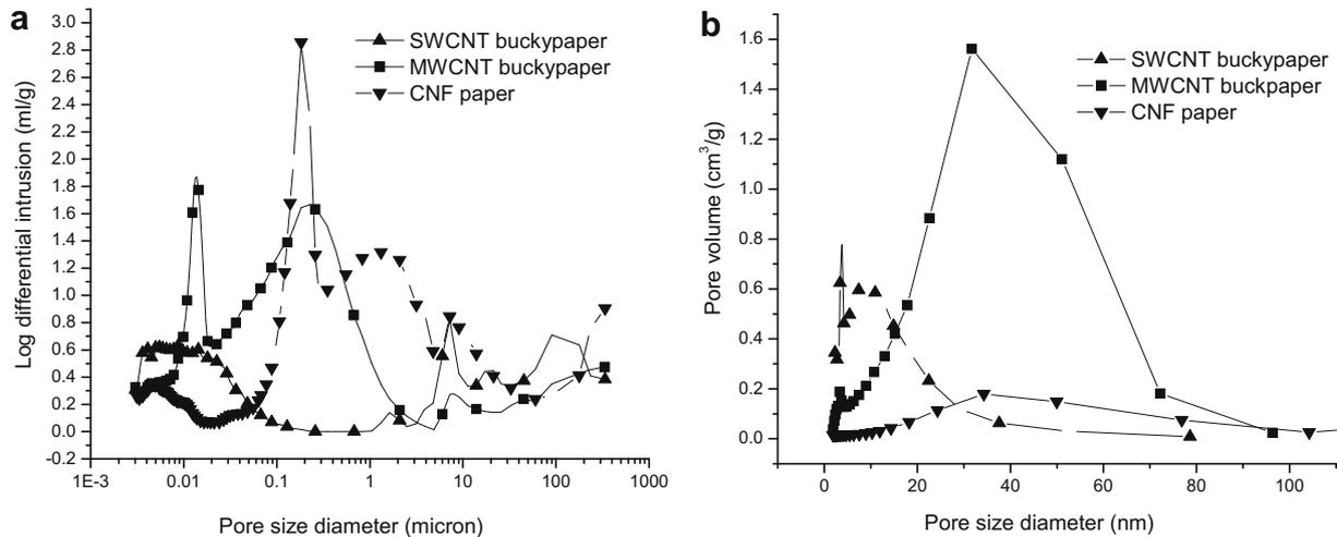
**Fig. 2 – Pore structures of SWCNT, MWCNT buckypaper and CNF paper. (a) Pore size distributions from mercury intrusion porosimetry. (b) BJH pore analysis of the buckypapers and CNF paper.**
