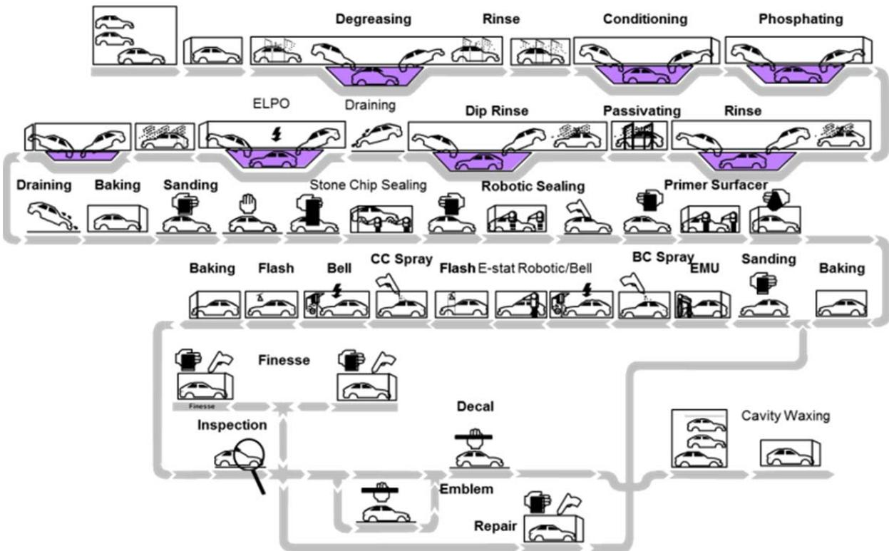
Figure 3 – Product Flow in Paint Process
