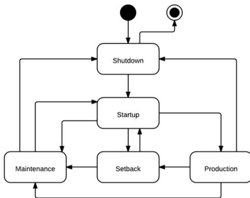
Figure 4 – UML State Diagram of Paint System Operating States
